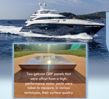
This project looks at accurately measuring the gelcoat surface quality and validating these various techniques. The study's results will benefit the marine industry to improve the design and manufacture of more efficient composite structures.
