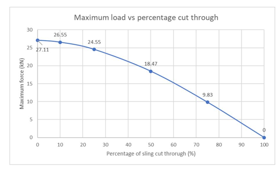
Cutting part way through the sling was found to have a smaller effect on the UTS than slight to moderate abrasion and a cut of 35% left the UTS above 22kN, whilst all abraded slings failed to meet this standard.
